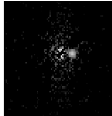
Figure 13: A simulation of the expected of an extrasolar planet. The simulation includes the effect of nulling, random and systematic wavefront error, amplitude and polarization mismatch, and photon and representative detector noise. In this simulation, two images are obtained with the planet at two different position angles (180 degrees apart) and then subtracted to remove the stellar leakage.
