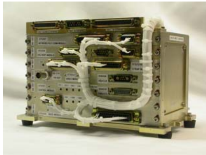
Figure 18: Left – The University of Wisconsin ST5000 Lost-in-Space star-tracker records stars down to 8 th mag in a field of 7.°1 x 4.°4. Right – The ST5000 electronics and computer with stored all-sky catalog.
