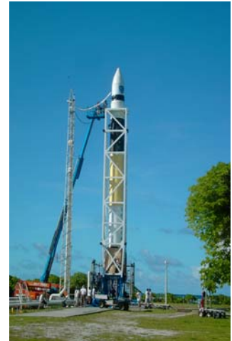
Figure 16: Top - The Falcon 1 vehicle installed on the launch pad at Omelek island. This was for the third mission F1-003. The elevated platform is being use for installation of electrical umbilicals and a duct used for payload environment control. Bottom – The Falcon 1 and 1e performance curves.
